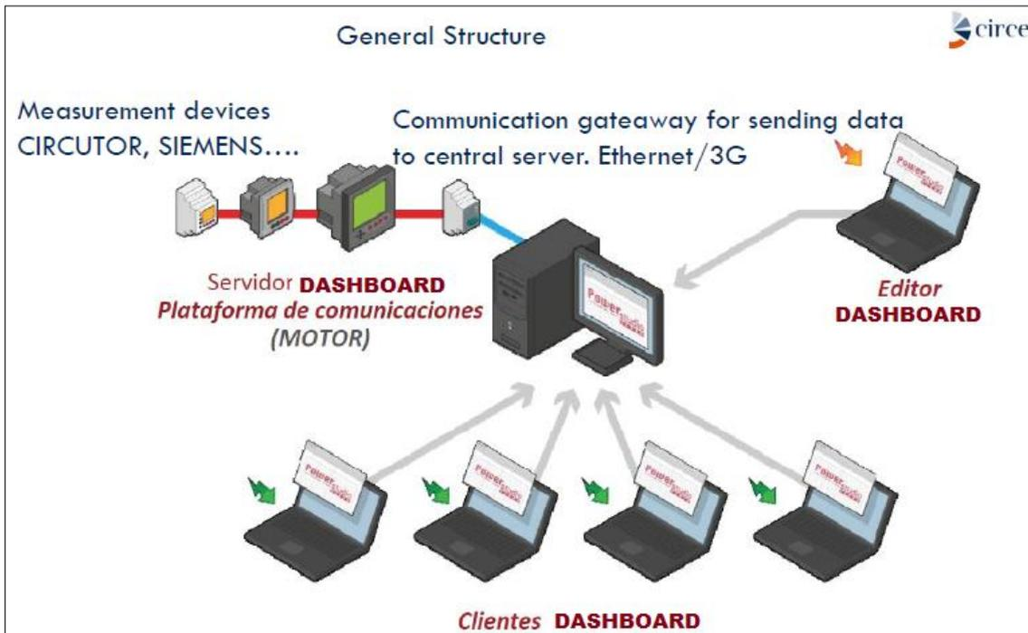
**Figure 2. General structure of the energy consumption monitoring and management system implemented in the clusters.**
